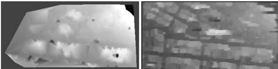
Fig. 4 Small section 400\text{ m} \times 200\text{ m} from an Ikonos-Scene of Athens (acquired 2004), left, DSM derived using the classical approach; right, DSM derived using a simple dense stereo approach
