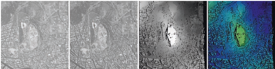
Fig. 20 Section 1 \times 1 km 2 , Athens, Acropolis, satellite image Ikonos, 24 July 2004, left and right stereo image, height map and color-coded and shaded height map
