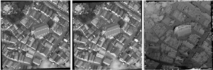
Fig. 19 Section 400 \times 400 m 2 , Vaihingen city center, left/center, left and right stereo image; right, derived height map
