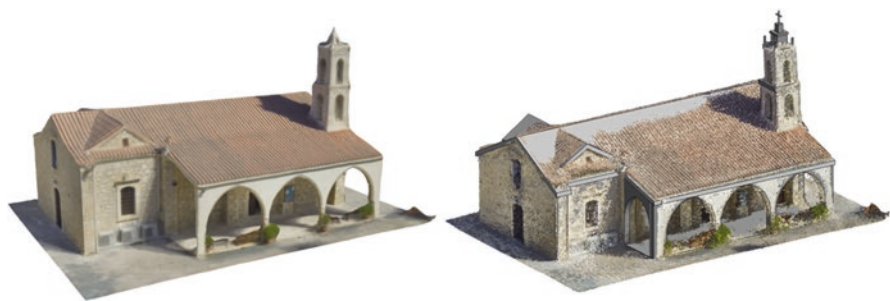
Fig. 20 Left, 3D model of church; right, 3D point cloud model integrated with BIM model
