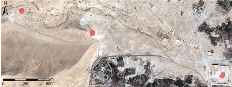
Fig. 7 Red: Post-processed change map from Fig. 6 overlaid on the 2nd of September 2015 WorldView-2 image reported in Fig. 5. All the main damaged areas are correctly identified (European Space Imaging/DigitalGlobe)
