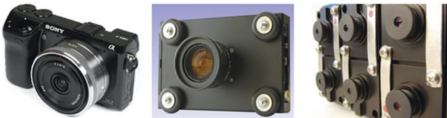
Fig. 1 Left—Sony NEX 7 visible spectrum camera. Center—Tetracam multispectral camera. Right—FLIR thermal camera
