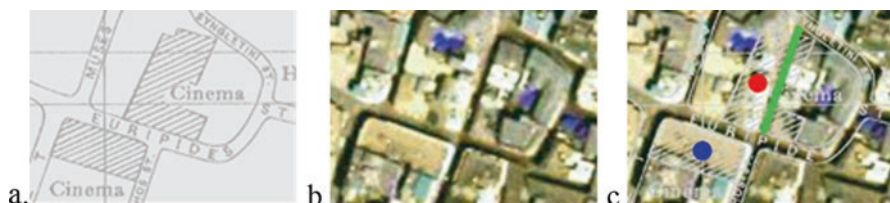
Fig. 9 Comparison of geographical data. (a) Map of 1956, (b) QuickBird-2 2006, (c) overlay: blue circle, a preserved building; red circle, a demolished building; green line, a new road
