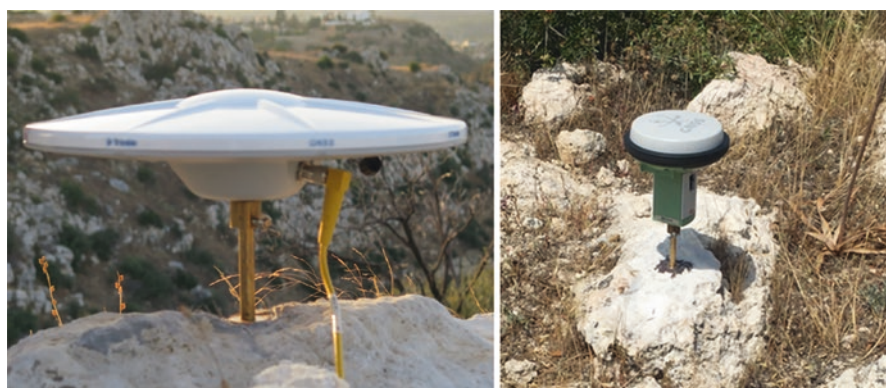
Fig. 8 Trimble Zephyr 2 GNSS (left) and Leica GS15 Smart GNSS Receivers (right) for establishing a GNSS control network
