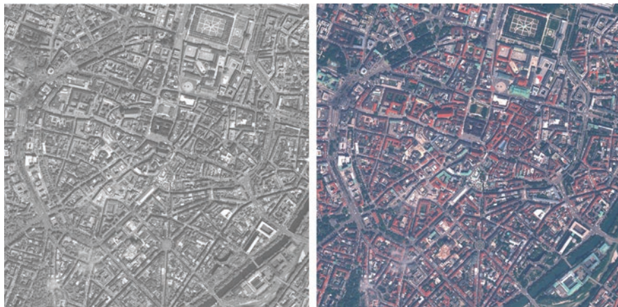
Fig. 16 Section 1.75 \times 1.75 km 2 , Munich city center, left, panchromatic “left” image; right, multispectral (red, green, blue) “left” image
