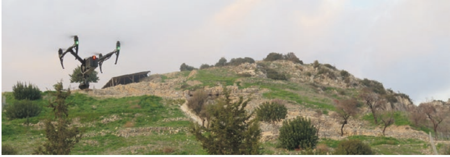
Fig. 24 Inspire 2 UAV with 20mp Zenmuse X5S camera and sensors
