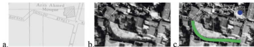
Fig. 8 Comparison of geographical data. (a) Map of 1956, (b) aerial photograph of 1963 in scale 1:5400, (c) overlay: inside the blue circle, there is a preserved building and with a green line, a new road
